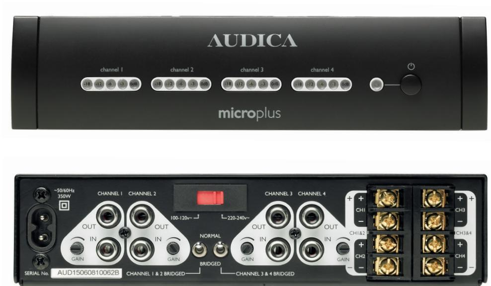
The Audica Professional MICROplus is an ultra-compact 4-channel power amplifier with the same size and style of head-unit mounting as the MICROzone pre/amp/controller; which it is designed to partner. It delivers 4 x 80W into 4 Ohm per channel, 2 x 80W into 4 Ohm plus 1 x 160W bridged into 8 Ohm or 2 x 160W into 8 Ohm with twin channels bridged.
