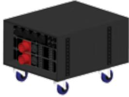
Anya's electrical power and signal distribution system is nearing completion, with design sketches for the 230 volt version shown here. Each unit will supply power for up to 12 modules and fully redundant Dante™ network for 12 modules. The rolling cases will stack or fly near the array to shorten cable runs.
